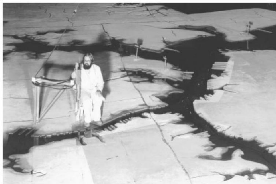
Chesapeake Bay Model technician at a tide gauge located on the Elizabeth River, at Portsmouth, Virginia, August 1977. U.S. Army Corps of Engineers Waterways Experiment Station photo
